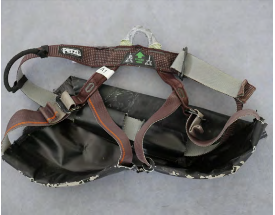
Figure 11: harnais A1 (2017) rupture du pontet à 18.84kN
