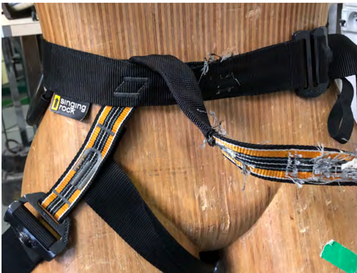
Figure 41: Harnais Singing Rock (SG2). Rupture de la cuisse à 18kN.
