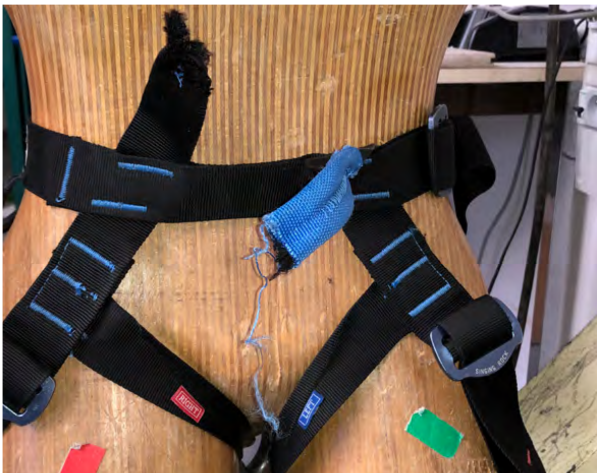
Figure 42: Harnais Singing Rock (SG3). Rupture pontet à 21.5kN.
